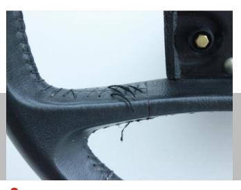
As you stitch, the edge of the leather may protrude. Use the larger sail needle to poke and press the edges down. It you run out of thread, or it snaps, you can knot a joint and make sure the knot is poked behind the seam.
