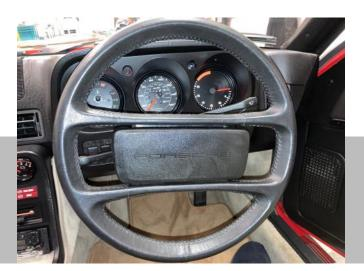
Once done, reattach the wheel to the car remembering to align the splines with your marks. Torque the nut tight (holding the wheel with your knees) and reattach horn wire and pad (this needs a firm even press to avoid snapping plastic fittings.
