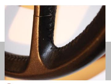
5 Measure the section you will repair and cut a length of the cotton four times as long (to allow for the stitch pattern). This way you'll not need to join the thread midway through, making it weak.
