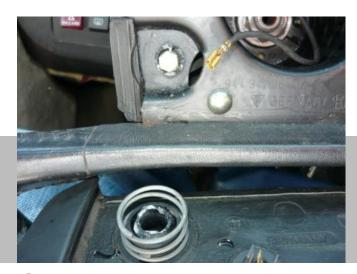
2 Remove the horn pad. It "simply" pulls off. Apply even pressure not to snap the locating pegs. Once free don't yank it away as you need to disconnect the horn wire. Mark the 12 o'clock position on the spline.
