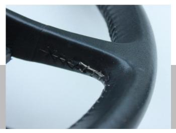
4 Inspect the wheel. If the leather needs repairing or re-dying then now is the time. Check what stitching you will replace. It is far better to do this in complete sections than to patch up small repairs. The inexpert "repairs" the precious owner did here didn't last... (yes it is string)
