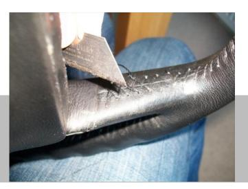
7 Decide the starting point so your eye won't see the starting stitch. Using a very sharp knife, cut a few of the existing threads and remove them with the pliers. No going back now! Only slice through a few threads at a time as it will keep the skin taut on the wheel.
